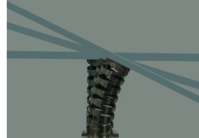
Fig. 8 Deformation of 6 V-shape units prototype piece under different loads shows the effectiveness of this type of continuum arm.
