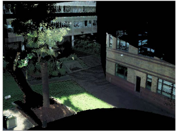
Fig. 1. A lidar's point cloud with a camera's image projected onto it.
