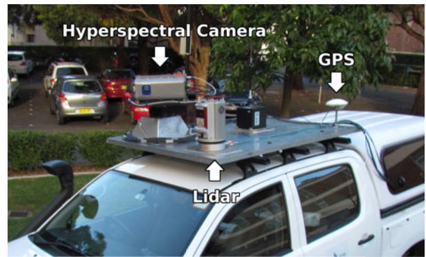
Fig. 6. Setup used to collect ACFR data
