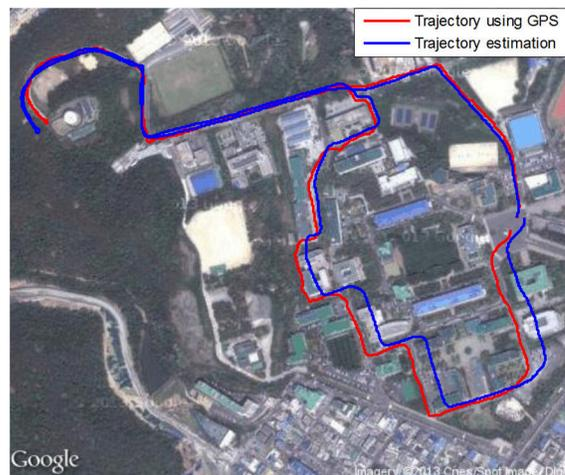
Fig. 9. Travelling localization estimation in long-distance
