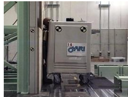
Figure 7. Collision between a six-year-old dummy in front of a wall and a mobile robot with a polystyrene panel. Robot mass, 200 kg; velocity, 6 km/h.
