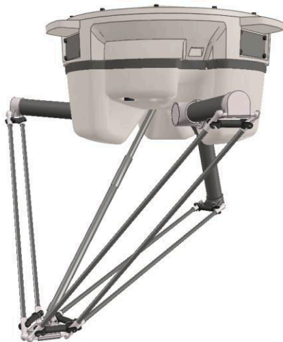
Figure 5. Delta Arm manipulator model in V-REP
