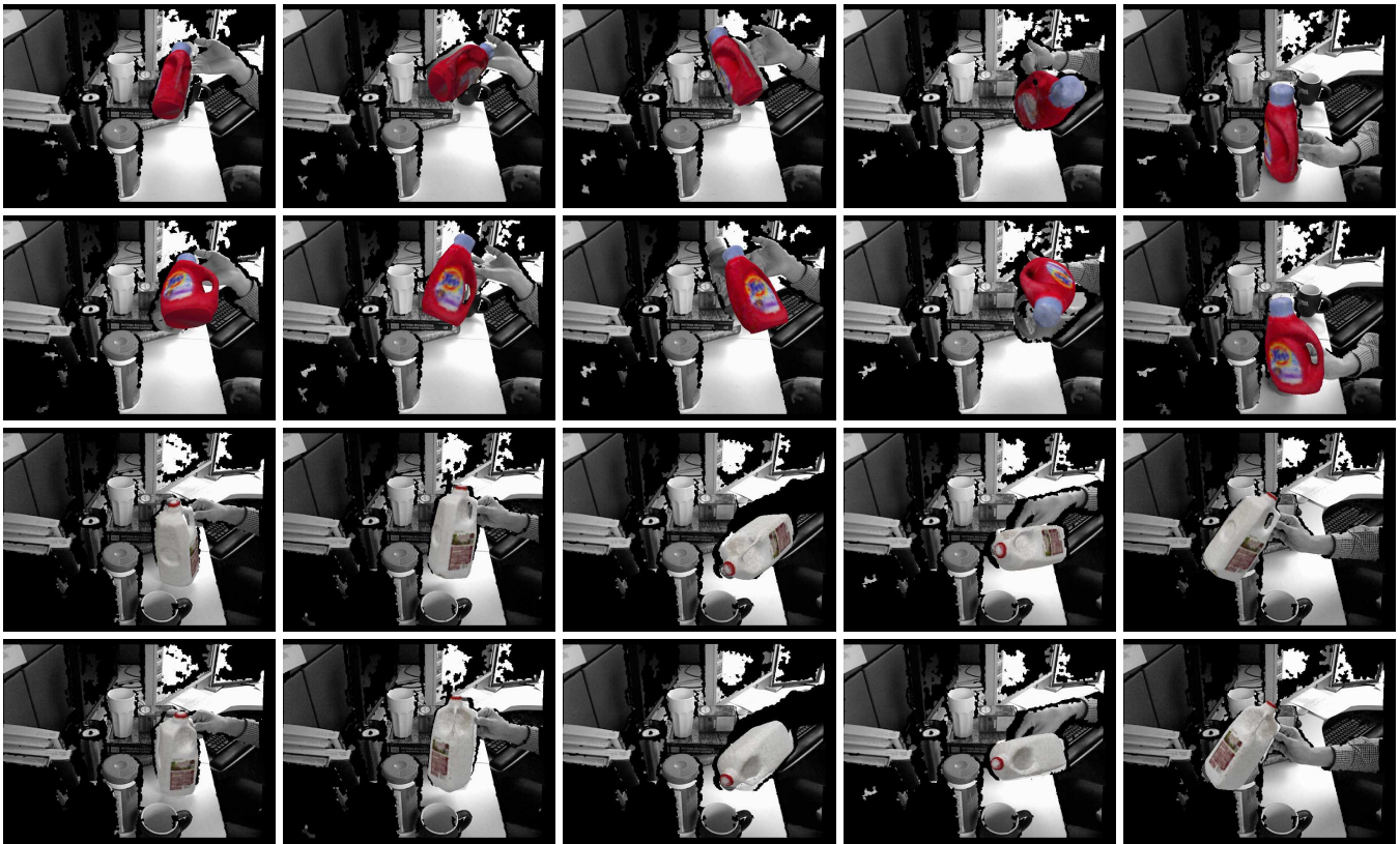
Fig. 7. Tracking results on the ‘Tide’ and ‘Milk’ real sequences. For both sequences, the upper rows show the tracking results of our approach, while the lower rows present the results of the PCL tracking ( N = 1600 ). As the objects undergo significant variations in rotations, the PCL tracking suffered from false pose estimates. Thanks to multiple model renderings every time, our tracking reliably tracks the true poses of the objects. (Best viewed in color)
