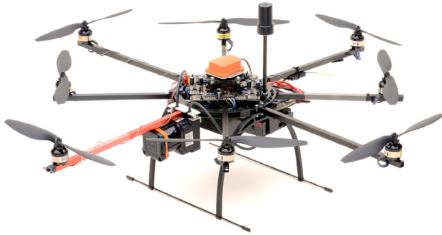
Fig. 1. The experimental flying platform with mounted GNSS-antenna and -receiver, laser scanner, IMU and processor-board.
