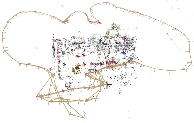
Fig. 4. Visualization of the map obtained by applying our proposed system on the freiburg3 dataset: Keyframe poses (red), edges between keyframes (golden), and map points (in their original color).
