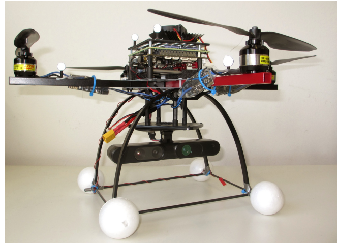
Fig. 1. The RGBD-UAV used for this work.
