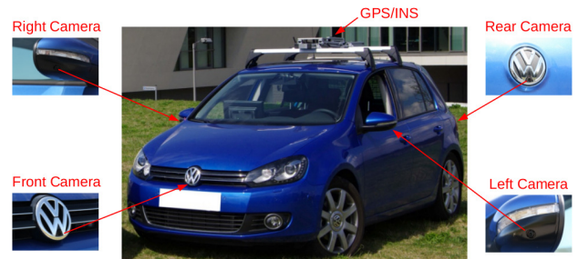
Fig. 1. Our car equipped with a multi-camera system with minimal overlapping field-of-views and GPS/INS system for ground truth.
