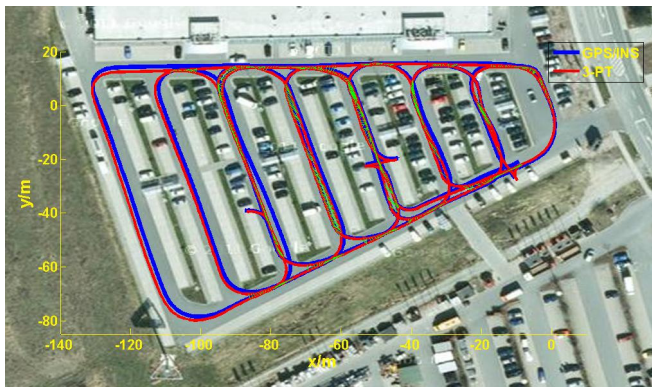
Fig. 9. Pose-graph for ParkingGarage02 dataset after pose-graph optimization (red) compared with trajectory from GPS/INS (blue) overlaid on the satellite image.
