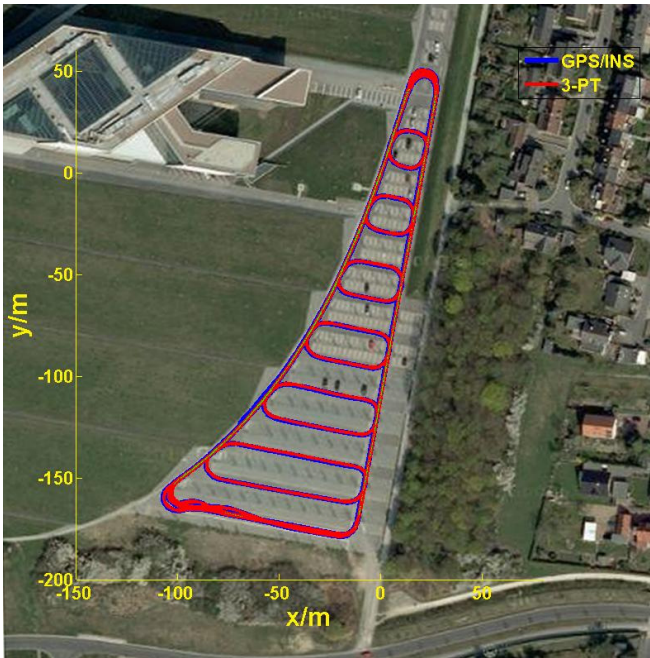
Fig. 7. Pose-graph for ParkingGarage01 dataset after pose-graph optimization (red) compared with trajectory from GPS/INS (blue) overlaid on the satellite image.
