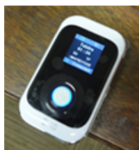
Fig. 9. Telstra Wi-Fi modem ZTE MF91. Two modems were used during the trial to connect with a public 3G network in Jindabyne.
