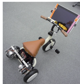
Fig. 1. Tricycle-style operation interface developed to allow young children to remotely control a robot [12], [13].
