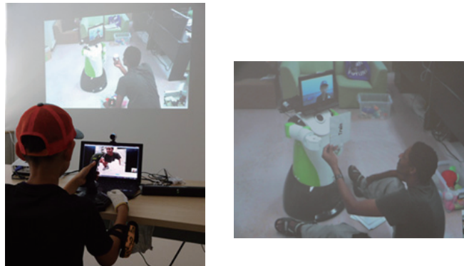
Fig. 2. Joystick and data glove (left image) to remotely control a robot (right image) placed in a remote location. The operator child is participating in a lesson given by an adult teacher (right image). Even if the operator cannot have a fluent conversation with a teacher speaking a different language, he/she can continue communicating with the teacher through the physical movement of the robot.
