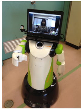
Fig. 3. Telepresence robot used in the study. It was based on Robovie-R3, which is commercially available from Vstone Co., Ltd [14]. To convert the base platform into the telepresence robot, a tablet PC and a monitor camera were mounted on the neck. Using Skype, the operator's face was projected on the monitor screen of the tablet PC. The right hand was fixed in the forward position, and only its opening/closing movement could be remotely controlled. The robot base could move forward, backward, right, and left.
