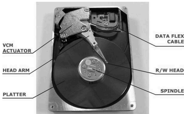
Fig. 1: View of typical components of HDD[15]
