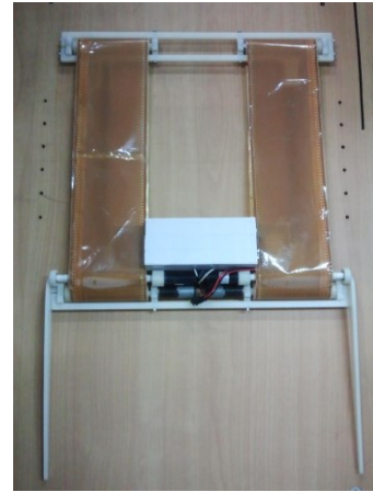
Figure 5. A double tracked wall climbing robot prototype.
