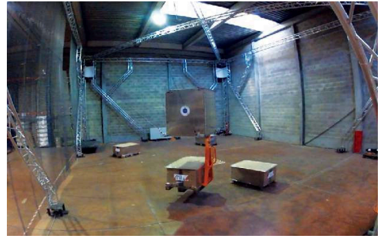
Fig. 2. The LIRMM/Tecnalia COGIRO suspended CDPR prototype.
