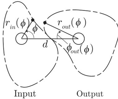
Fig. 5. Design method of pitch curve
