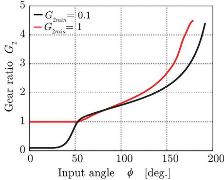
Fig. 7. Gear ratio of non-circular gears
