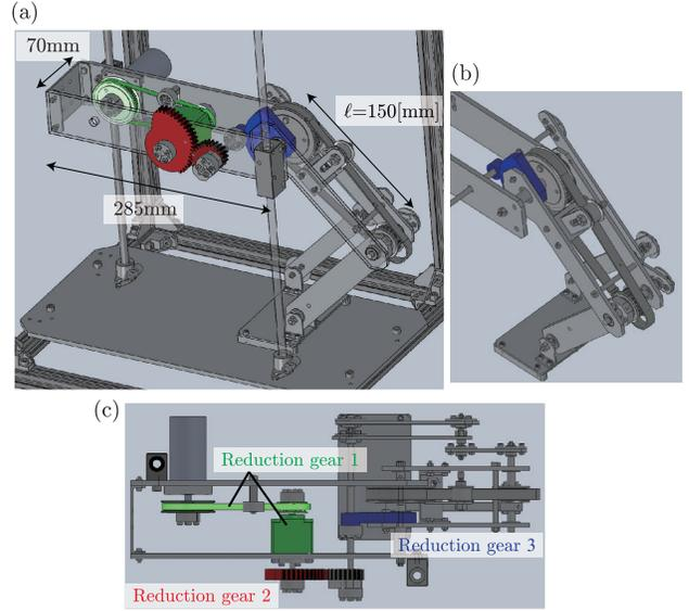
Fig. 6. Design of jumping robot
