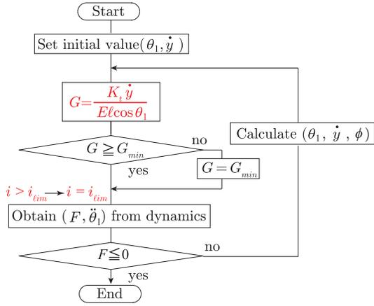
Fig. 3. Design of optimal change of gear ratio with simulation-based method
