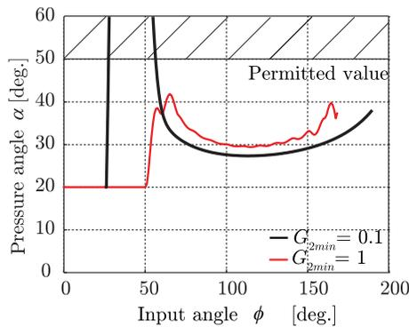
Fig. 9. Operating pressure angle
