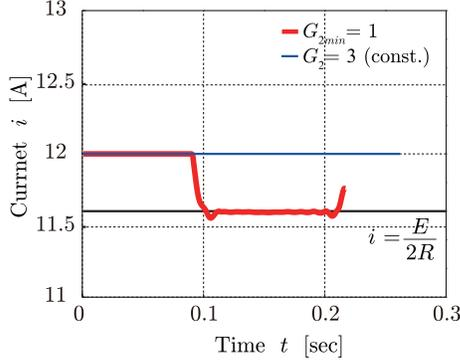
Fig. 13. Current value of the motor in jumping motion
