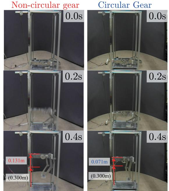
Fig. 15. Experiment of jumping robot with non-circular gear and with circular gear
