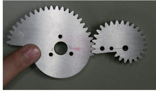
Fig. 10. Prototyped non-circular gear
