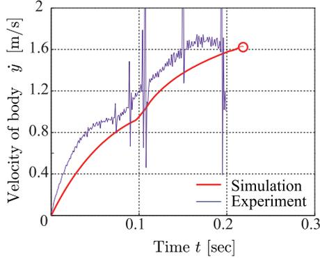
Fig. 16. Experimental result of of body velocity of the robot
