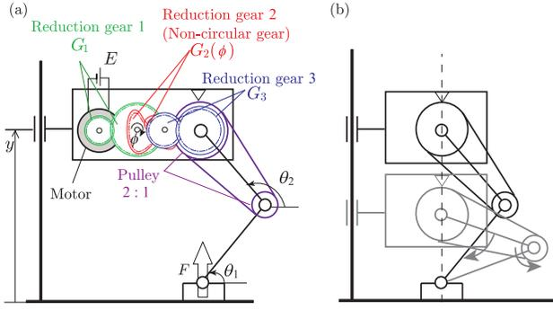
Fig. 2. Jumping robot with a non-circular gear
