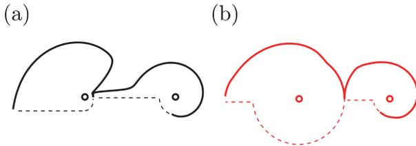
Fig. 8. Pitch curves of designed non-circular gears
