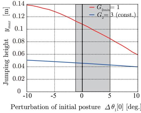
Fig. 12. Jumping height with respect to perturbation of initial posture
