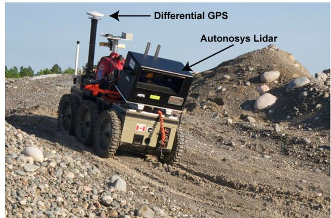
Fig. 1. This figure shows the ROC6 rover, equipped with an Autonosys LVC0702 lidar and a Thales DG-16 Differential GPS unit.
