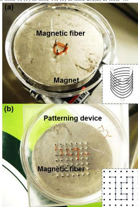
Fig.10 Manipulation of magnetic hydrogel fiber with magnetic tweezers system. (a) coiling magnetic hydrogel fiber on three steel pillar; (b) aligning magnetic hydrogel fiber on a patterning device.
