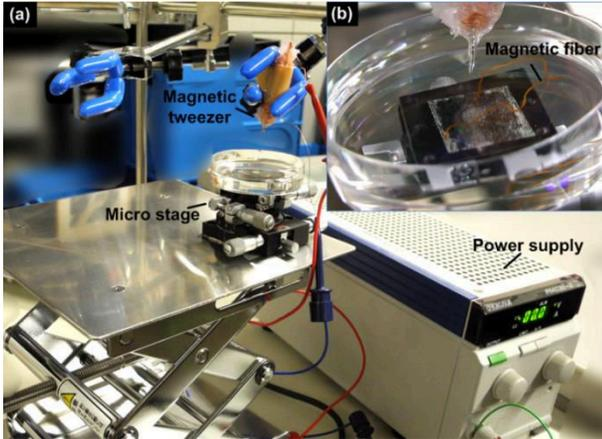
Fig.5. Magnetic tweezers system based on electromagnet. The magnet consists of a single coil enclosing a soft iron core. The core is needle shaped at the end, the magnetic flux is then bundled and the magnetic field reaches a maximum near the tip. (a) device structure; (b) enlarged view of magnetic tweezers.
