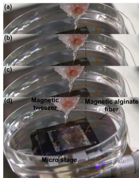
Fig.9. Experiments for manipulating magnetic alginate fiber at different time.(a) at time 0; (b) at time 1s; (c) at time 2s;(d) at time 4s.
