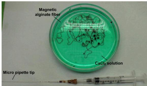
Fig. 4 Injection of magnetic alginate solution for solidification. A syringe is connected with a micro pipette for achieving magnetic fiber with small diameter of 0.8mm.
