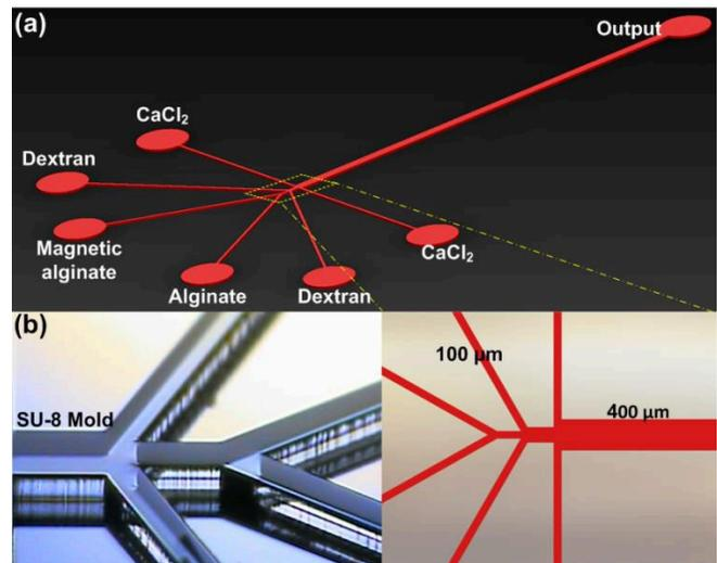
Fig.2. Illustration of the fluidic chips used in the fabrication of magnetic hydrogel fiber. (a) Pattern design of microfluidic chips with the exact size; (b) SU-8 mold used for fabricating microfluidic device.
