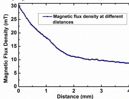
Fig.8. Magnetic flux density as a function of distance from the tip of magnetic tweezer.
