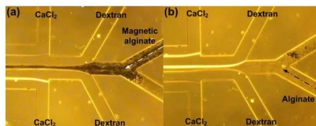
Fig. 6. Illustration of laminar flow at the central area of the fluidic chip during the fabrication of magnetic hydrogel fiber. (a) Input of magnetic alginate.(b) Input of nonmagnetic alginate.
