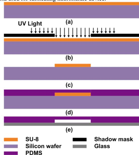
Fig.3. Fabrication process for the microfluidic device. (a) SU-8 was spin-coated on the silicon wafer; (b) UV light exposure under specific shadow mask; (c) SU-8 model was achieved after development; (d) PDMS was spin-coated on the SU-8 mold; (e) Peeling off the PDMS from the wafer and bonding it on the cover glass.
