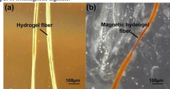
Fig.7. Optical image of hydrogel fiber. (a) Nonmagnetic hydrogel fiber; (b)magnetic hydrogel fiber.
