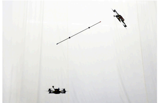
Fig. 1. Illustration of two quadrocopters passing a pole between them. The right quadrocopter throws the pole towards the left vehicle, which tries to catch and re-balance it.
