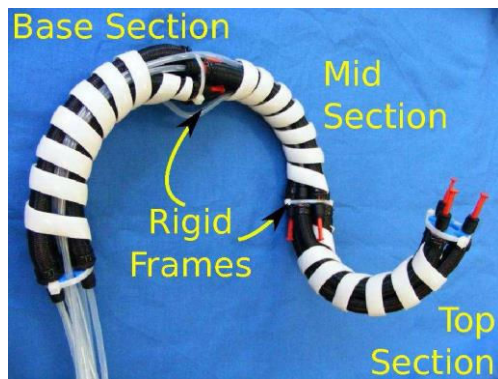
Fig. 9. Third generation arm prototype: bending in air
