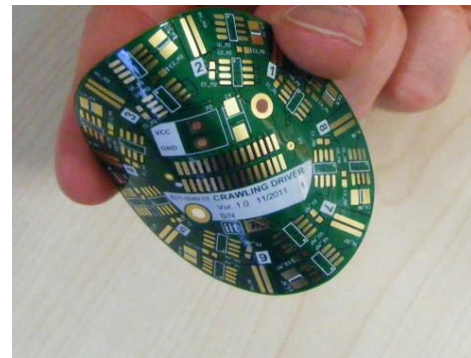
Fig. 4. Flexible circular shaped electronic board
