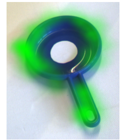
Fig. 2: Projection of a 6D grasp density onto a 2D image. For more details we refer the reader to the work of Detry et al. [10].
