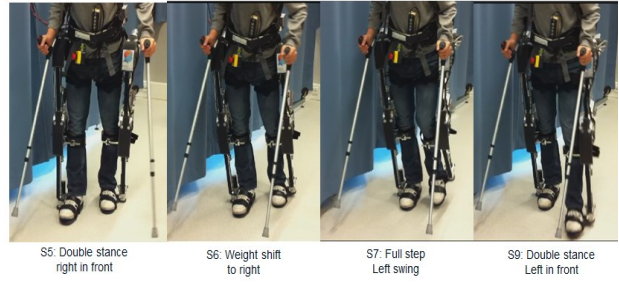
Figure 8. A snapshot of a left step during the straight walking. The crutches were only used as safety protection and didn't touch the ground during the whole procedure.
