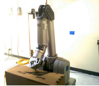
Fig. 1: Whole Arm Manipulator (WAM) feeling an obstacle boundary.
