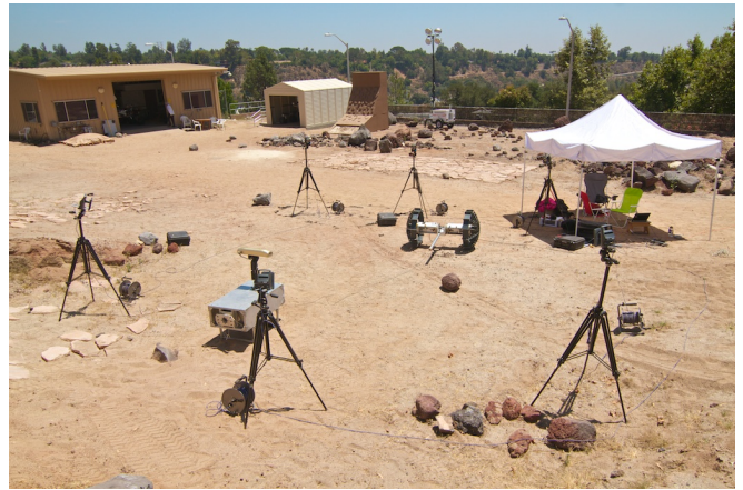
Fig. 8: Autonomous docking experiments with the VICON ground truth system in the JPL Mars Yard.
