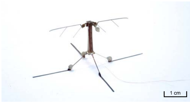
Fig. 7. Photograph of the robotic insect with extended landing gears. The extensions are attached to the current structure through a viscoelastic urethane material.
