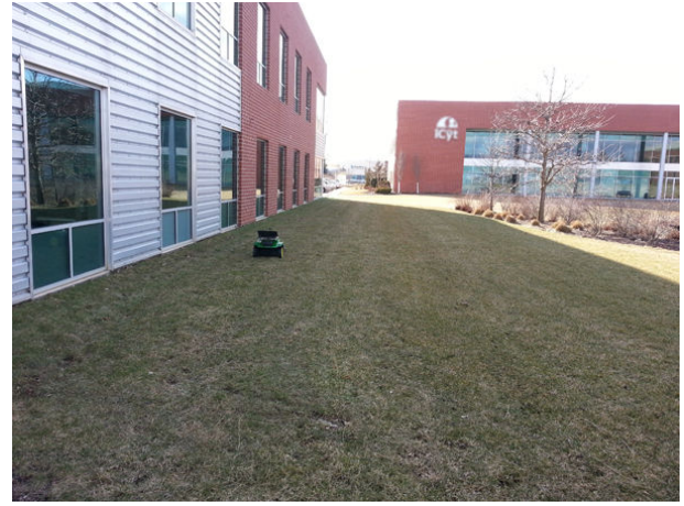
Fig. 9. Our autonomous mower following a boundary set-up in the backyard of our research building for map estimation and boundary teaching
