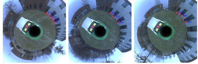
Fig. 10. Tracking landmarks in a sequence of omnidirectional camera images
