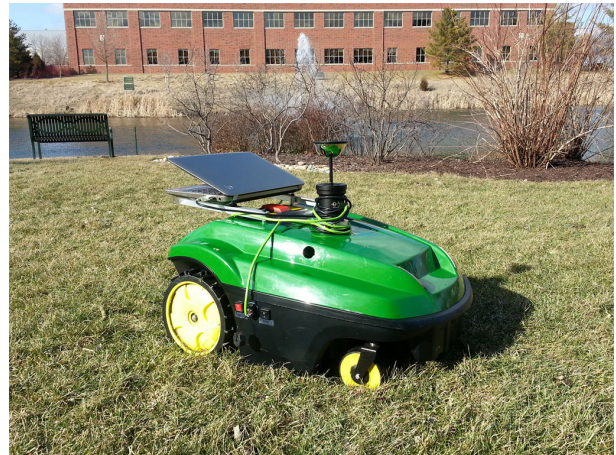
Fig. 1. Our autonomous mower modified with an omnidirectional camera and an IMU for experiments
