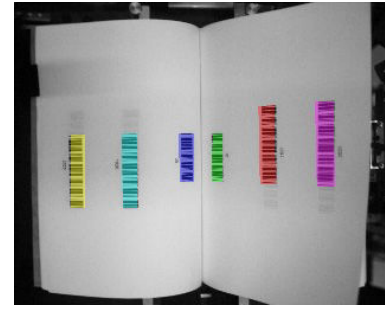
Fig. 15. Examples of the detected barcodes on the page.
