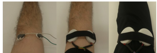
Figure 5. Electrode placement methods: standard vitrode, hybrid electrode resistive mode, hybrid electrode capacitive mode
