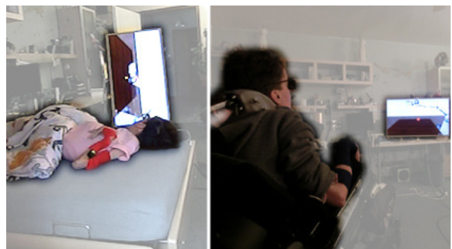
Fig. 4. Participants SH and SV equipped with sEMG electrodes and shutter glasses, while controlling the robot simulation on a 3D-monitor. One participant preferred to lie down during the experiments, whereas the other participant preferred to control the robot sitting in the wheelchair.
