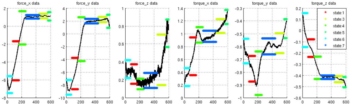
Fig. 5. Learned segmentation for a wrench time-series of  $step_4$  of execution scenario *nominal*. The different colours correspond to different values of  $z_t$  and the horizontal lines represent the  $2\sigma$  interval of the corresponding Gaussian emission parameters. Plots for wrench first order derivatives are omitted.
