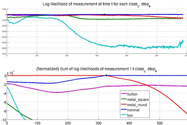
Fig. 7. (top) Plot of  $\log p(\mathbf{w}_{s_t} | \Pi_{class_c})$  and  $\log p(\mathbf{w}_{s_1:s_t} | \Pi_{class_c})$  (bottom) for  $step_4$  of a nominal execution trial. From  $t > 325$ , the log-likelihood of all the measurements from  $s_1$  to  $s_t$  is constantly highest for the nominal class.
