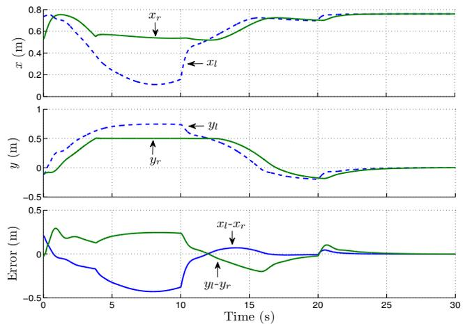
Fig. 6. Cartesian local and remote positions and Cartesian position error when interacting with a stiff wall.
