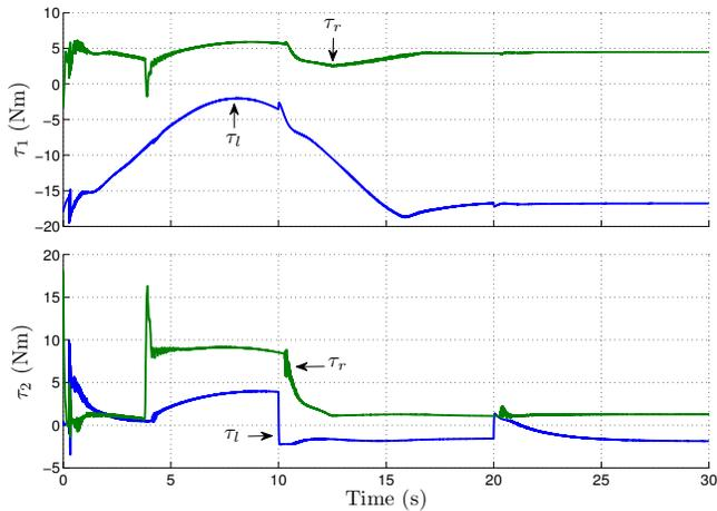
Fig. 7. Local and remote controller torques when interacting with a stiff wall.
