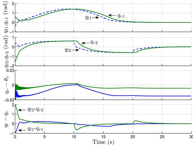
Fig. 3. Articular position and error for the local and remote manipulator.
