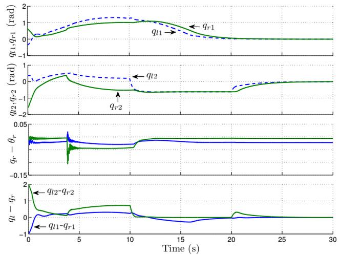
Fig. 5. Local and remote articular position and error when interacting with a stiff wall.
