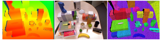
Fig. 1. Raw depth image (left), color image (middle) and resulting 3D object segmentation (right).
