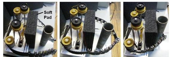
Fig. 8. Grasping stages of a cylindrical object with a diameter of 50mm
