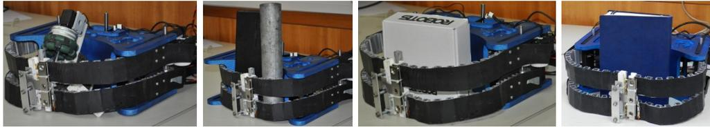
Fig. 14. Flexirigid gripper could adapt to a variety of object profiles due to its flexibility and could successfully grasp them. Images show the status of the gripper before and after retraction of the trunks.
