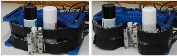
Fig. 16. Two different approaches for grasping two objects. The second approach (right picture) is by active control of each trunk to form it close to the object's profile.
