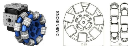
Fig. 14. Design of the 4<sup>th</sup> generation of magnetic wheels.
