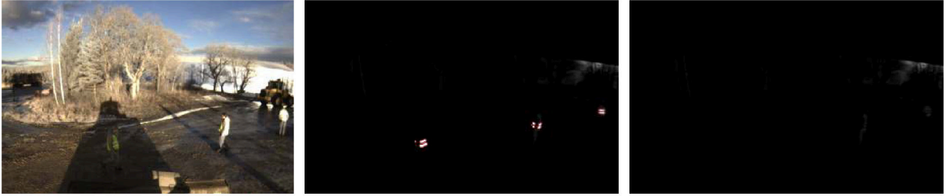
Fig. 3. Outdoor scene containing a total of 3 persons (left) with corresponding input images as captured by one of the NIR cameras using IR flash (center) and without using flash (right). Reflective regions as identified in the segmentation process are indicated with a red contour.
