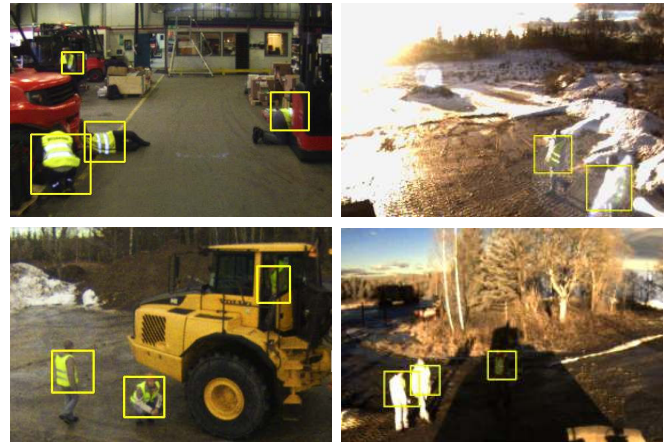
Fig. 1. A selection of challenges faced by human detectors in industrial work environments, including partly occluded workers in non-upright body poses as well as varying illumination settings. Detections as obtained from our human tracker are indicated with yellow squares.
