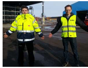
Fig. 9. The two types of reflective safety clothing used throughout the experiments: ANSI/ISEA safety class 2 vest with reflectors only around the body (right) and safety class 3 jacket with additional reflectors in the shoulder and arm area (left).
