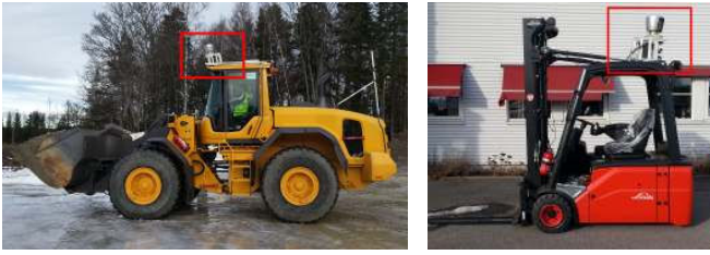
Fig. 7. Wheel loader (left) and forklift (right) on which the camera setup was evaluated. The location of the sensor unit is indicated in red.
