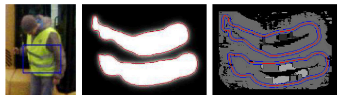
Fig. 5. The figure illustrates how disparity is computed for a detected blob: The scene (left) is captured with the NIR camera and the resulting image I_f (middle) is segmented to extract the contours of the reflectors, drawn in red. A disparity map (right) is then computed in the neighborhood of each contour by using the images I_f of both NIR cameras. Due to the lack of texture, disparities are sometimes not (black pixels) or erroneously (differing gray levels) computed in regions within the blob. However, consistent results are obtained from the regions near the contour and therefore only the zone delimited by blue lines is taken into consideration.
