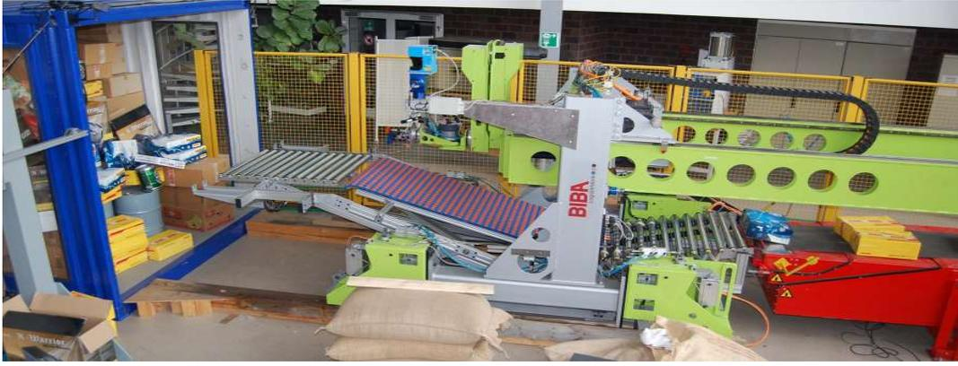
Fig. 3. The set-up of the RobLog scenario for container unloading.
