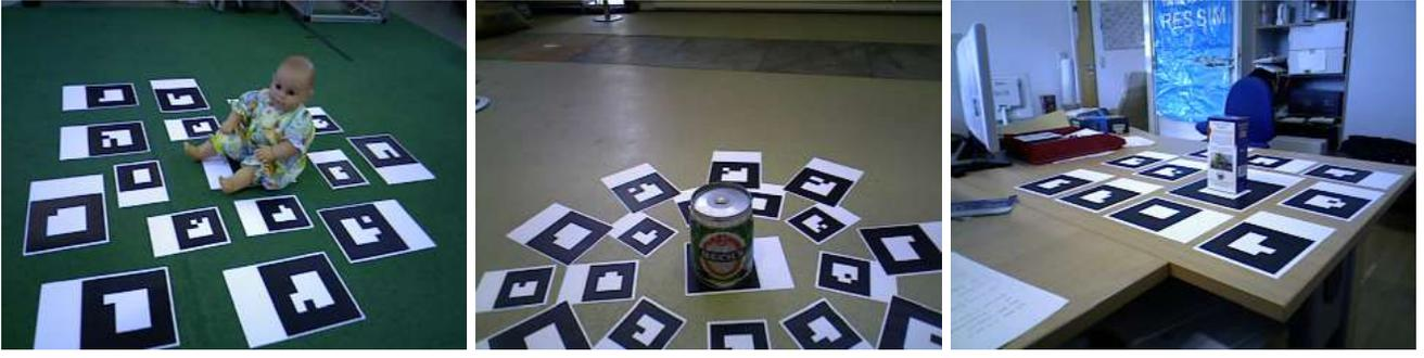
Fig. 4. The Augmented Reality (AR) markers that provide coarse localization information can be freely placed in the scene where the object is recorded. This allows the modeling of objects of very different sizes.
