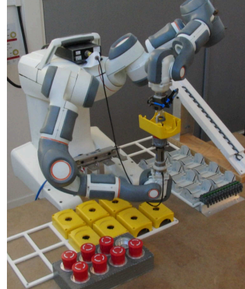
Fig. 1. The setup for the assembly task used in the experiments. The force/torque sensor, mounted at the wrist of the robot's right arm, is only used for verification and evaluation of the estimated forces.
