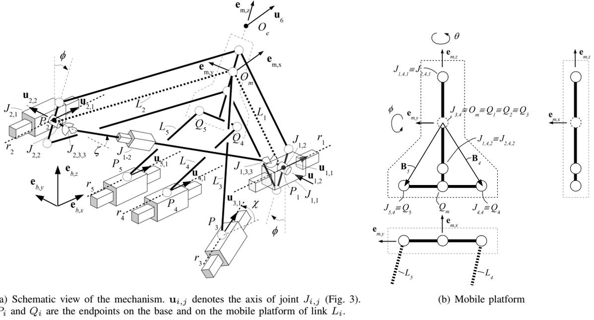
Fig. 2. Vectorial representation of the 5dof partially decoupled 3T2R parallel kinematic architecture.
