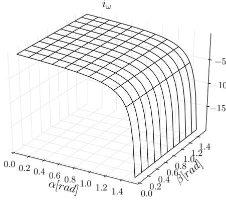
(a) Linkage angular velocity ratio with  $\gamma = 0$
