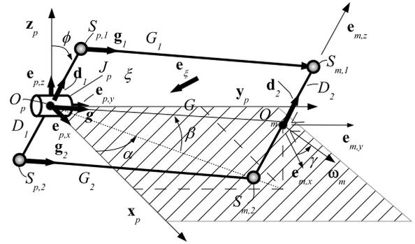
Fig. 5. The four-bar linkage
