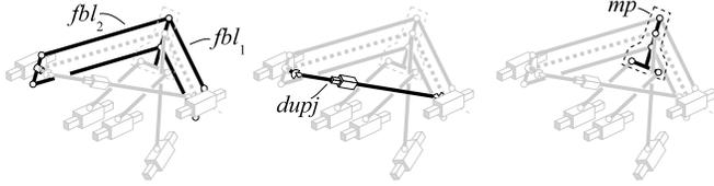
Fig. 4. Mechanism subsystems are denoted by  $fbl$  (four-bar linkage),  $dupj$  (double universal prismatic joint) and  $mp$  (mobile platform).
