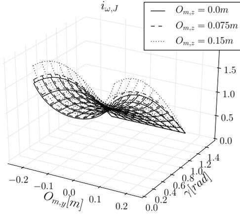
Fig. 8. Relative angular velocity between  $J_{2,2}$  and  $J_{2,1}$ . Because of symmetry,  $O_{m,z}$  is evaluated only for positive values.
