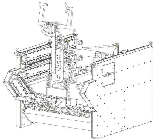
Fig. 1. The presented architecture constitutes the mechanical heart of the Active Headframe, a robotic prototype designed to actively support the patient's head in open-skull awake surgery.
