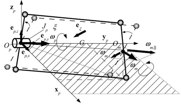
Fig. 6. Angular velocity transmission in the four-bar linkage.
