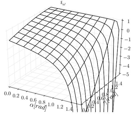
(b) Linkage angular velocity ratio with  $\beta = 0$
