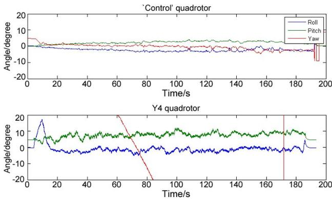
Fig. 10: Quadrotor Outdoor Flight Roll, Pitch and Yaw Angles.
