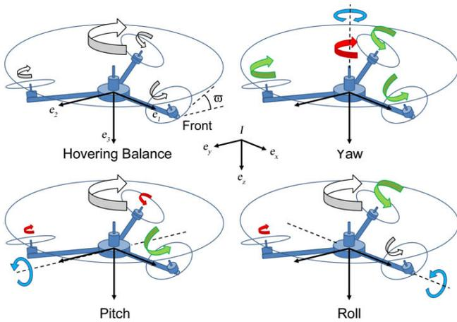
Fig. 2: Triangular Quadrotor Manoeuvring Controls. Arrow sizes indicate relative rotor velocities (white arrows are constant).
