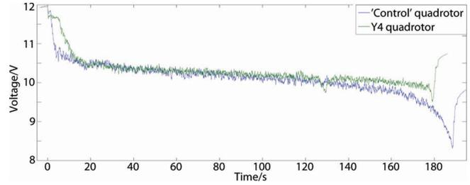
Fig. 8: 'Control' and Triangular Quadrotor Battery Voltage in Flight.
