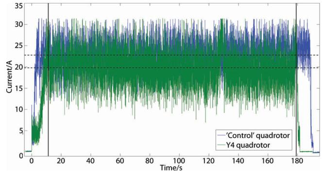
Fig. 7: 'Control' and Triangular Quadrotor Current Draw in Flight.
