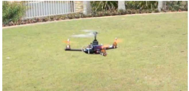
Fig. 9: Triangular Quadrotor Hovering Outdoors.
