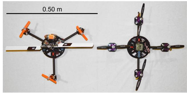
Fig. 5: Y4 Triangular Quadrotor and ‘Control’ Standard Quadrotor.
