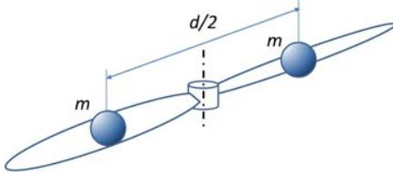
Fig. 4: Two-Point Mass Rotor Inertia Model.
