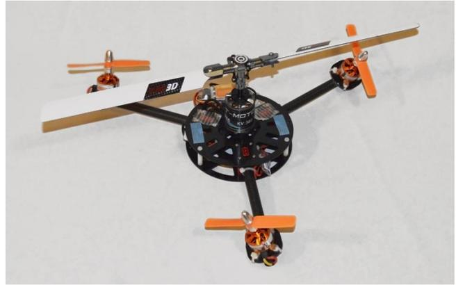
Fig. 1: 'Y4' Triangular Quadrotor Configuration.
