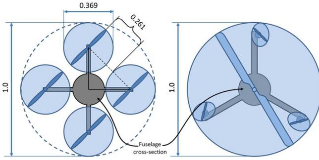
Fig. 3: Conventional Quadrotor and Triangular Quadrotor Rotor Spacing and Lifting Area Comparison — Unit Diameter Footprint.
