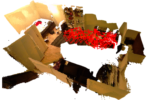
Fig. 1. Room B sequence. A raw point based model generated using the SLAM mode. The apartment is scanned using a RGB-D sensor by hand in a single 360° sweep. The result is not a photorealistic 3D model and memory consumption becomes high.
