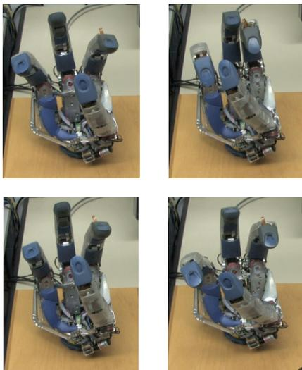
Fig. 4. In the first row (left initial position, right final position) the first synergy mapped onto the DLR II hand using the s-IPC controller. In the second row the second mapped synergy.
