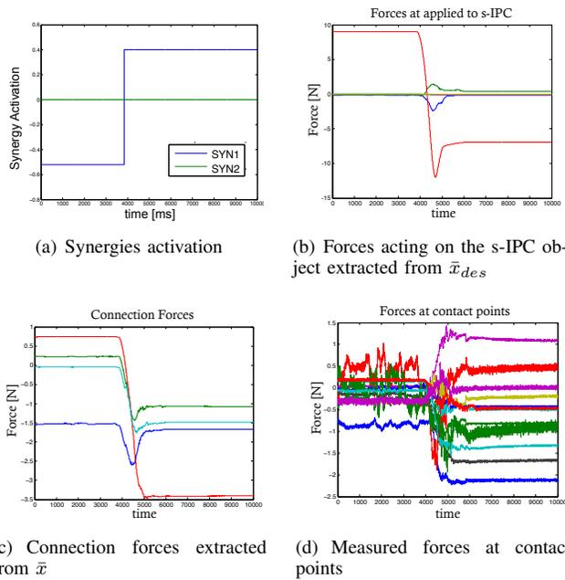
Fig. 6. Grasping a ball using the first mapped synergy and the s-IPC controller.
