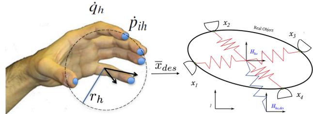
Fig. 1. The motion of the paradigmatic hand is described by the virtual sphere. The arising parameters  $\bar{x}_{des}$  are used as input for the s-IPC controller.
