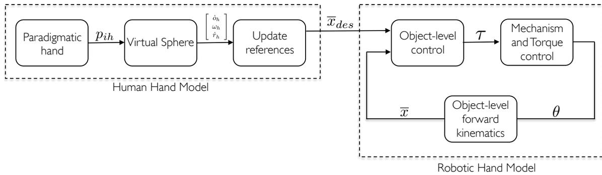
Fig. 3. Block diagram of the virtual sphere mapping plus the s-IPC. The task is performed by the paradigmatic hand model and reference signals are computed for the low level controller of the robotic hand, the s-IPC.
