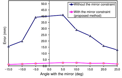
Fig. 10. Error in measurement of the marker position against the angle between the robot and the mirror
