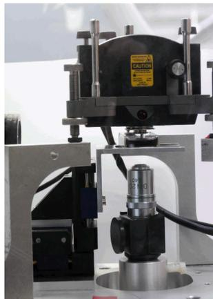
Fig. 10. AFM with substrate in liquid medium.
