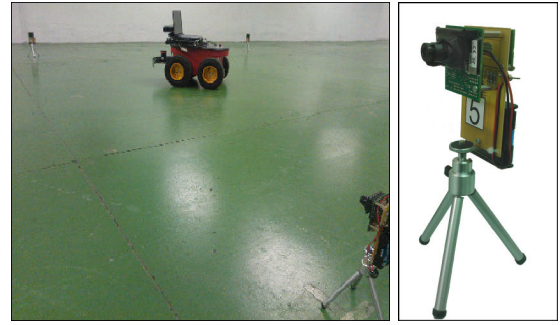
Fig. 4. Left) Picture of the CONET Integrated Testbed taken in the experiments. Right) Camera node used in the experiments.
