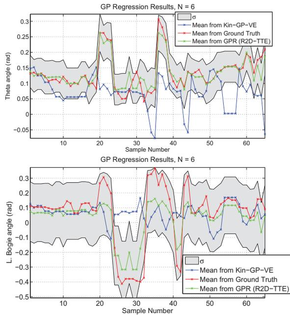
Fig. 10. GP regression results for predicting  $\theta$  and  $\alpha_1$ , respectively, over an area with higher deformation than that experienced during training. Grey area indicates a  $1\sigma$  confidence interval.
