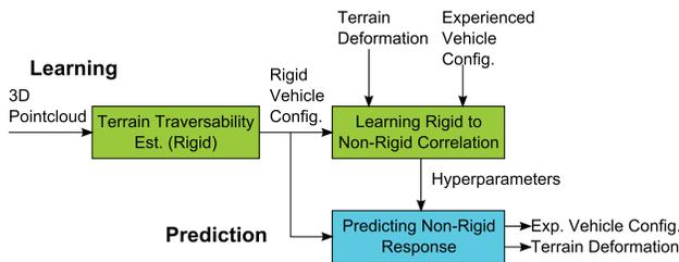
Fig. 4. System architecture for Rigid to Deformable Terrain Traversability Estimation (R2D-TTE)
