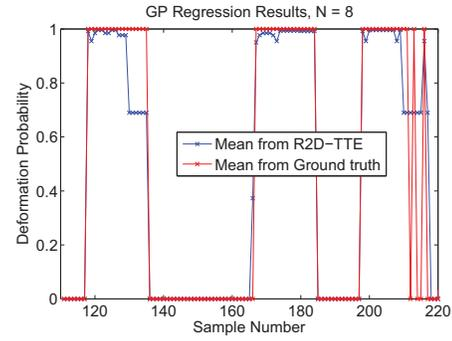
Fig. 8. GP regression results for predicting  $\mathcal{T}_{deform}$  over 500 validation points, zoomed over sample number 110 to 220.
