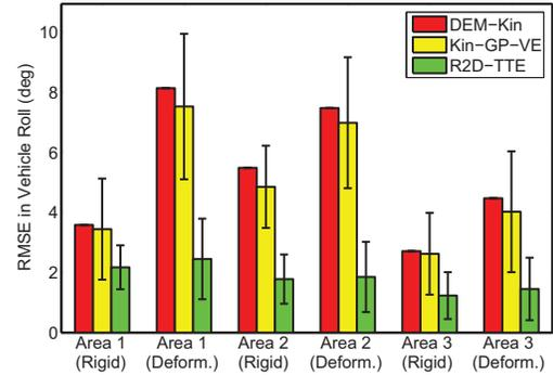
Fig. 9. RMSE in vehicle Roll from GP regression results for Kin-GP-VE and R2D-TTE
