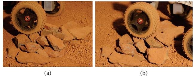
Fig. 1. Rover traveling over deformable terrain: (a) before traversal (front wheel); (b) during traversal (back wheel). Note the differences of rock configurations between (a) and (b).
