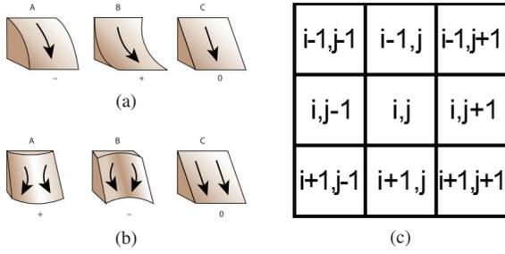
Fig. 5. (a) Profile Curvature. (b) Planform Curvature. (c) Cell reference of the vehicle position index  $(i, j)$  for determining  $\phi(i, j)$  on the DEM.
