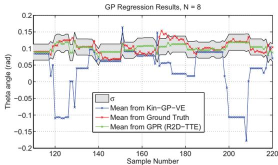
Fig. 7. GP regression results for predicting  $\theta$  over 500 validation points, zoomed over sample number 110 to 220. Grey area indicates a  $1\sigma$  confidence interval.
