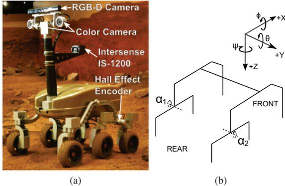
Fig. 6. (a) Mawson Rover. (b) Chassis Configuration.
