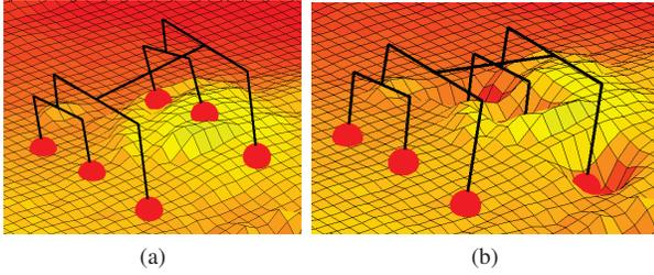
Fig. 2. Vehicle attitude in a simulation environment: (a) without terrain deformation, (b) with 10cm of terrain deformation. With terrain deformation, the vehicle experienced a change of 18° in roll and 10° in left bogie angle.
