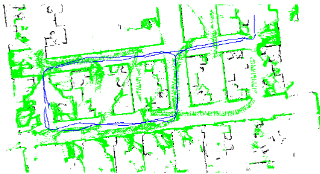
Fig. 9: Pose Map of Dataset 3 obtained using C-LOG with plot of all raw laser reading for each pose. The fact that the laser scans align well with the map demonstrates the accuracy of the localisation algorithm. The laser readings in the middle of the corridors depict people moving around the environment.
