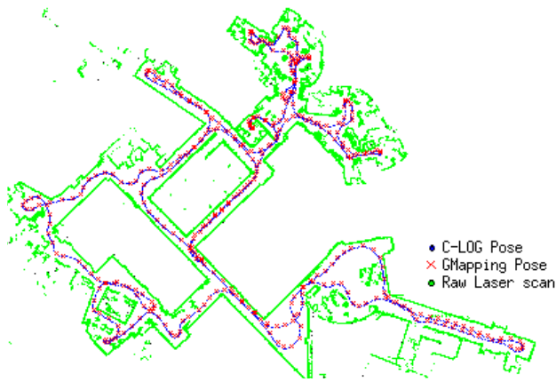
Fig. 8: Robot poses of C-LOG and GMapping with the occupancy grid map constructed using C-LOG poses for Dataset 2.
