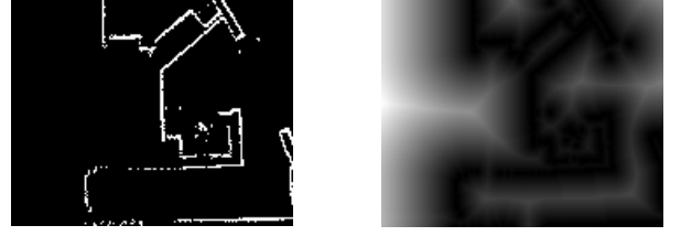
Fig. 1: (a) Map and (b) Distance Transform Image for a part of the Intel Research Labs Dataset
