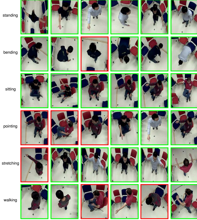
Fig. 5. Results of the posture recognition based on our top-view dataset. The example images are randomly sampled from the testing results. The text on the left indicates the ground-truth posture label of the images in the row. Postures that are correctly recognized are in green rectangles, and postures are in red rectangles if wrong labels are predicted.
