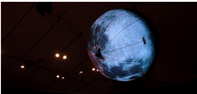
Fig. 12. Skye as the moon. A printed hull and internal LEDs enable nighttime aesthetic effects.
