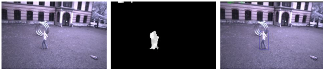
Fig. 14. Computer vision algorithm to detect a waving user. From left, one frame of a captured sequence, detected motion, detected rectangle of largest motion.
