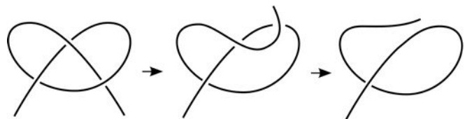
Fig. 9. Process of untangling a rope using a node deletion followed by a Reidemeister move.
