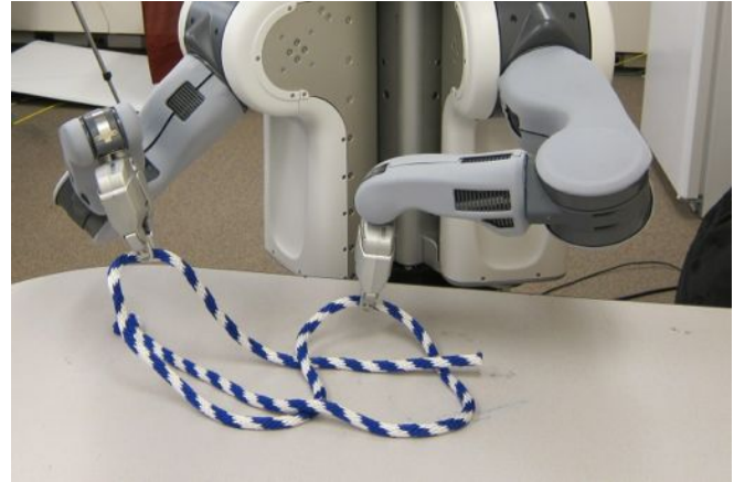
Fig. 1. Our robot observes a knotted rope using its RGB-D camera, infers its knot structure and chooses appropriate manipulation actions to untangle the rope.
