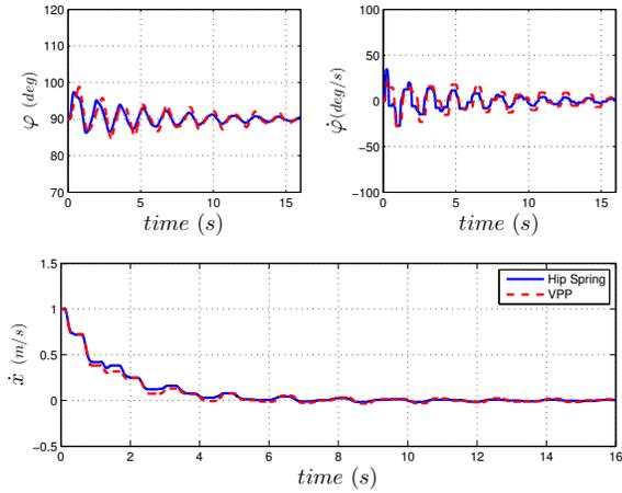
Fig. 3: Hopping response to 1  $m/s$  perturbation with hip spring and VPPC-FP.
