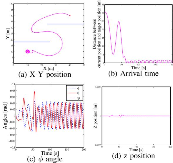
Fig. 9: Results with combining NADFs and clamping control
