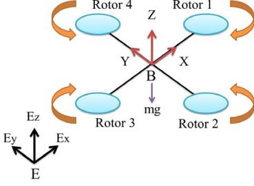
Fig. 4: Structure of the X4-Flyer and the definition of coordinates
