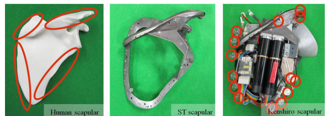
Fig. 7. Design of blade bone compared with human. It can be seen that the 3 dimensional shape for insertion is realized by the design.
